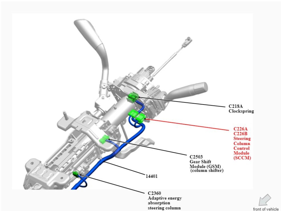
**Plug in the HSW connector behind the SCCM(C226B)**
